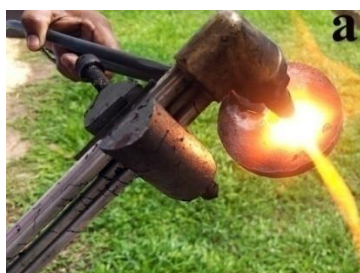
Carbon foam developed from waste newspaper exposed to oxyacetylene flame
