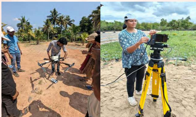
Figure: Students using drone and Hyperspectral imager for image acquisition in the field
