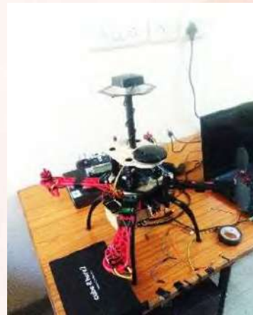
Figure: Magnetotorques and Single axis Momentum wheel based ADCS system developed at IIST by M Tech Control Systems students.
