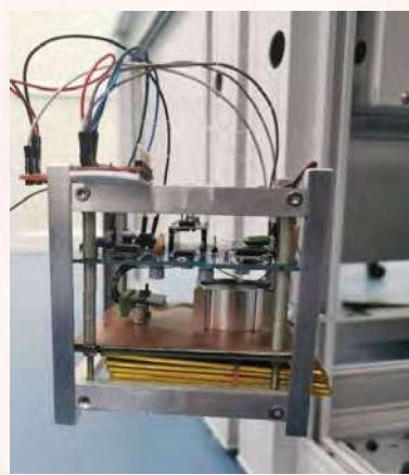
Figure: Magnetotorques and Single axis Momentum wheel based ADCS system developed at IIST by M Tech Control Systems students.
