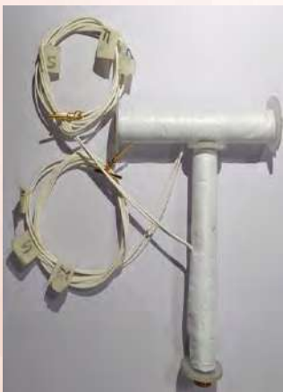
Figure: Magnetotorques and Single axis Momentum wheel based ADCS system developed at IIST by M Tech Control Systems students.
