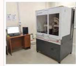
X-ray Diffractometer (XRD) Model: Anton Paar XRDynamic 500
