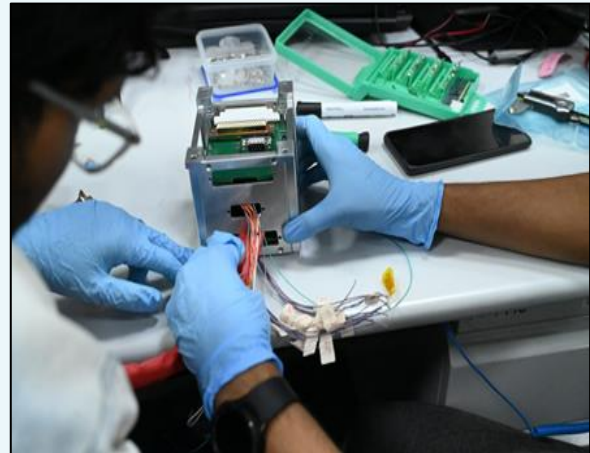
Routing the harness: every wire labelled, every connection deliberate
